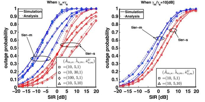
Fig. 2. The SIR distributions  $\mathcal{S}_{m,c}^U(T)$  and  $\mathcal{S}_{s,c}^U(T)$  in an HCN.
