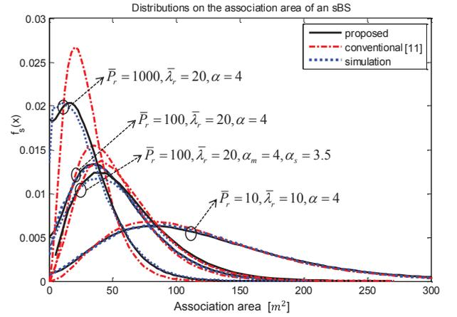
Fig. 2. The distribution on the association area of an sBS.
