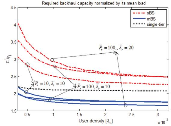
Fig. 5. The normalized required backhaul capacity for a BS in tier  $j$ .
