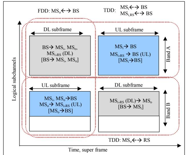
Fig. 2. Frame structure of overlaid HDD system.
