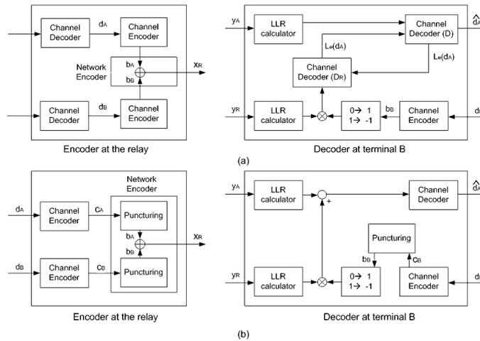
**Fig. 1.** Encoders and Decoders (a) re-encoded network coding scheme (b) flexible network coding scheme.
