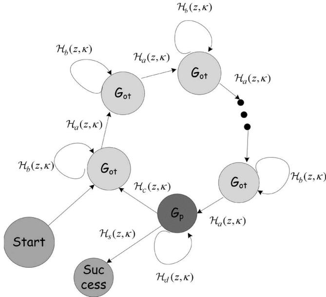
Fig. 4. Equivalent state-transition diagram for acquisition.
