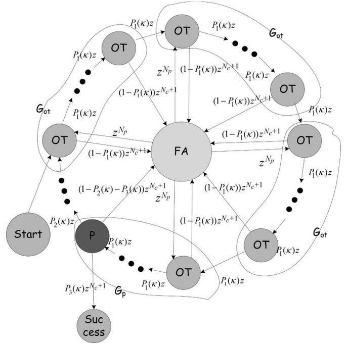
Fig. 3. State transition diagram for acquisition.
