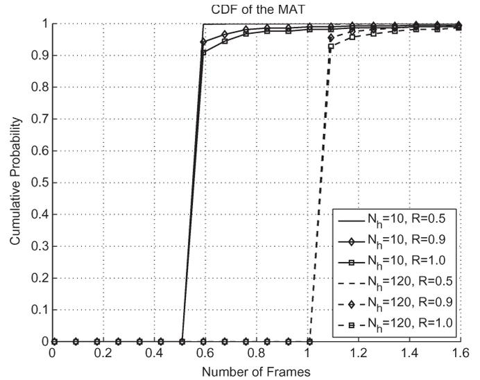
Fig. 9. CDF of the MAT in multicell environments.
