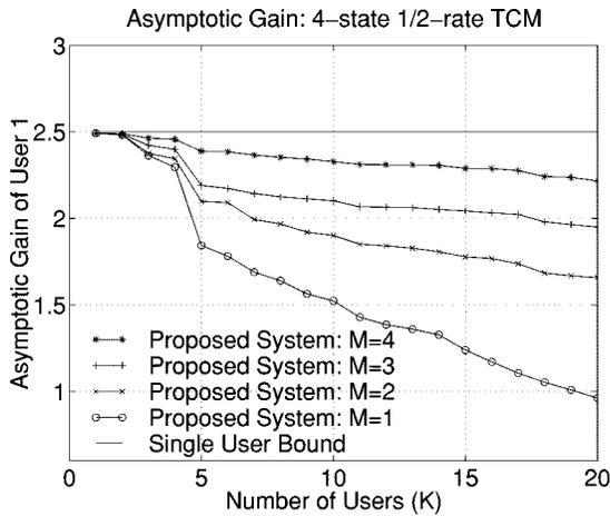
Fig. 7. Asymptotic gain of the proposed system with base-station antenna array with no interleaving.
