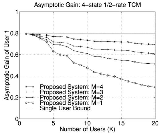
Fig. 8. Asymptotic gain of the proposed system with base-station antenna array with interleaving and perfect CSI.
