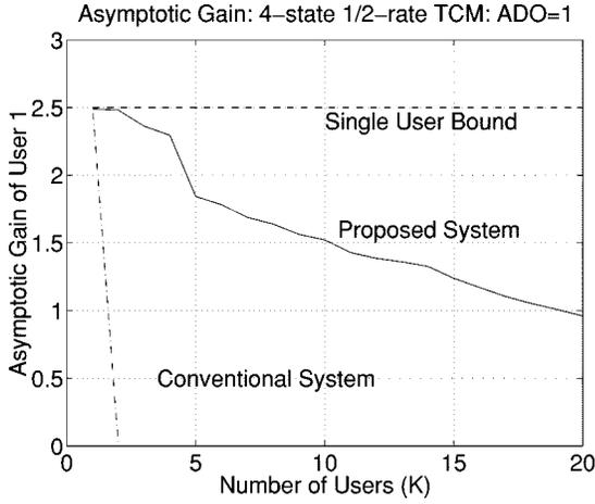
Fig. 3. Asymptotic gain of the proposed and conventional systems with no interleaving.
