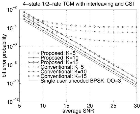
Fig. 6. Bit error probability bounds of the proposed and conventional systems with interleaving and perfect CSI.
