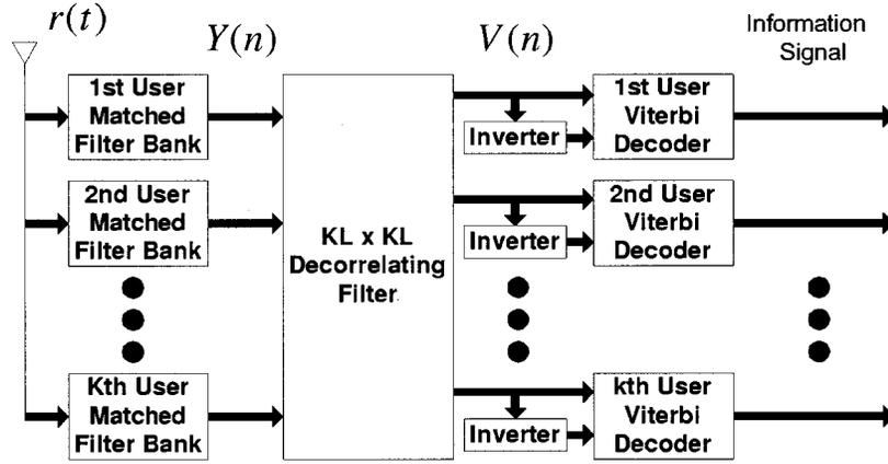
Fig. 2. The receiver structure of the proposed system.
