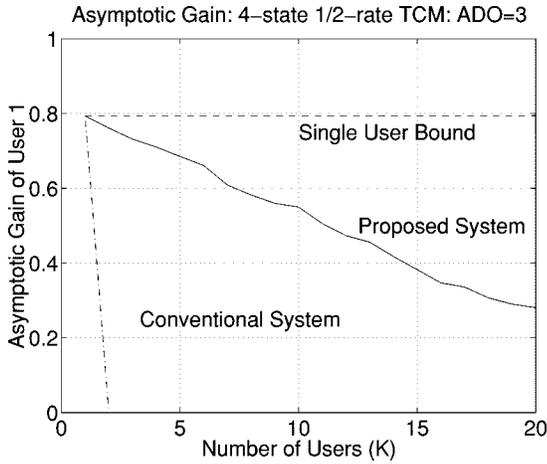
Fig. 5. Asymptotic gain of the proposed and conventional systems with interleaving and perfect CSI.
