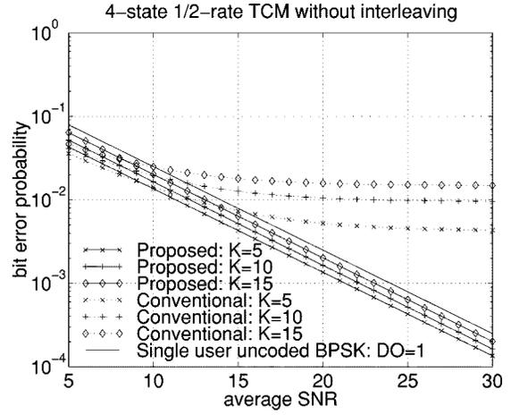
Fig. 4. Bit error probability bounds of the proposed and conventional systems with no interleaving.
