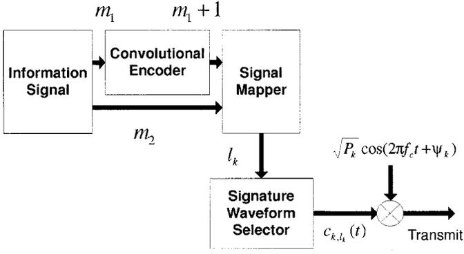
Fig. 1. Transmitter structure of the trellis-coded DS/CDMA system.
