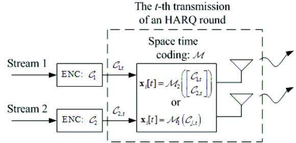
Fig. 1. The block diagram of the transmitting part of  $\mathcal{S}$  or  $\mathcal{R}$  at the  $t$ -th slot
