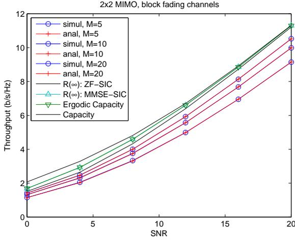
Fig. 2. The throughput of MIMO-HARQ without relay versus SNR
