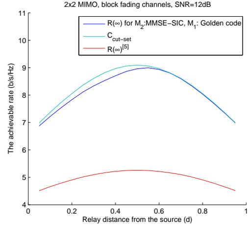
Fig. 3. The achievable rate of MIMO-HARQ protocol with relay and the cut set bound of the ergodic capacity
