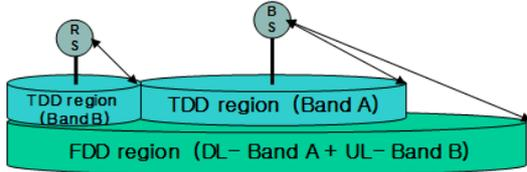
Fig. 2. Overlaid HDD system.
