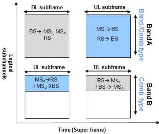
Fig. 4. Proposed frame structure for proposed overlaid HDD system.
