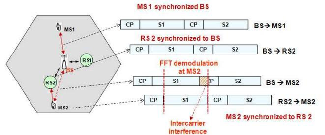
Fig. 5. Example of intercarrier interference.
