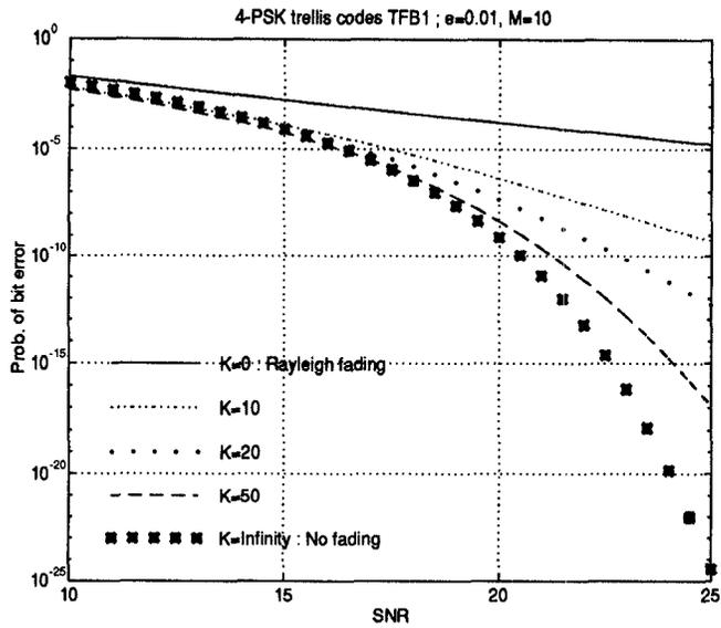
Figure 3: The bit error probability for various  $K$  when  $M = 10$  and  $\epsilon = 0.01$ .
