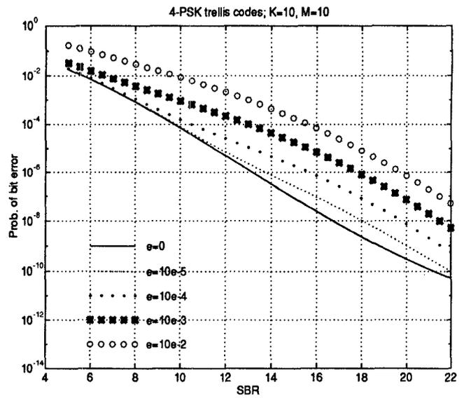
Figure 5: The bit error probability for various  $\epsilon$  when  $K = 10$  and  $M = 10$ .
