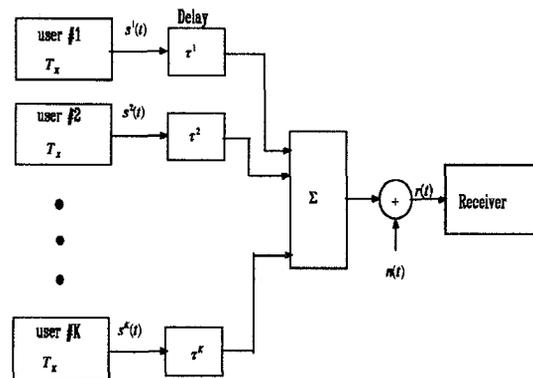
Figure 1: A block diagram of the general system architecture.
