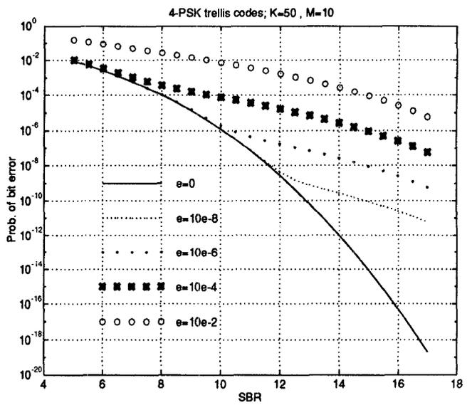
Figure 6: The bit error probability for various  $\epsilon$  when  $K = 50$  and  $M = 10$ .
