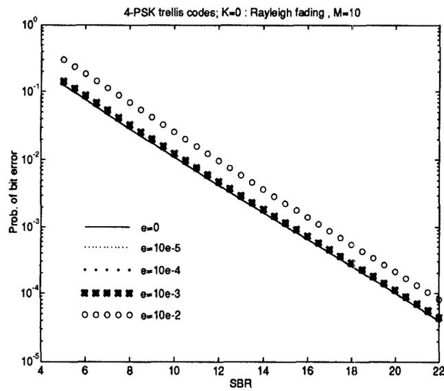
Figure 4: The bit error probability for various  $\epsilon$  when  $K = 0$  and  $M = 10$ .
