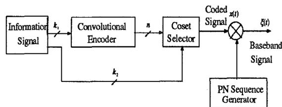
Figure 2: The transmitter system model for the trellis-coded DS/SSMA.
