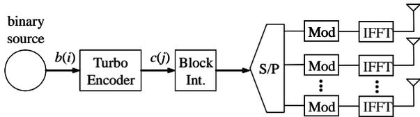
Fig. 1. Transmitter of turbo processing system
