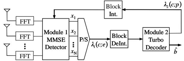
Fig. 3. Proposed turbo processing system with non-linear MMSE detector
