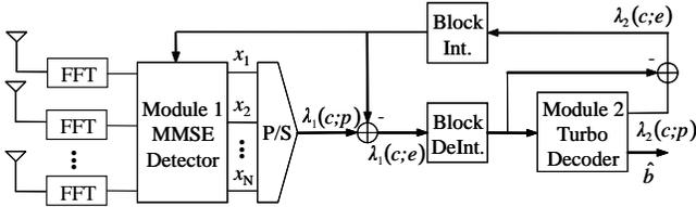
Fig. 2. Conventional turbo processing system with linear MMSE detector
