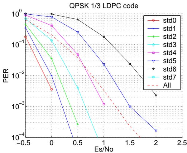
Fig. 3. The packet error probability of the MCS option using 4-QAM and 1/3-rate LDPC code.
