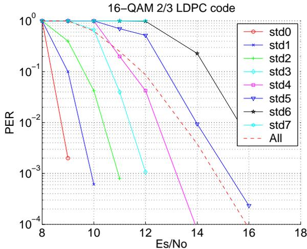
Fig. 4. The packet error probability of the MCS option using 16-QAM and 2/3-rate LDPC code.
