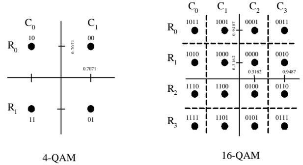
Fig. 2. The Gray encoded 4-QAM and 16-QAM constellations.
