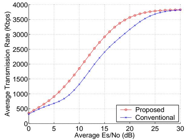
Fig. 5. The performance of the proposed adaptive transmission scheme.
