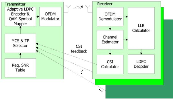
Fig. 1. The system model for the proposed adaptive transmission.
