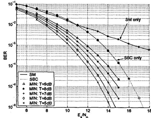
Figure 7. The BERs of the proposed system when the ML detector is employed for the SM.
