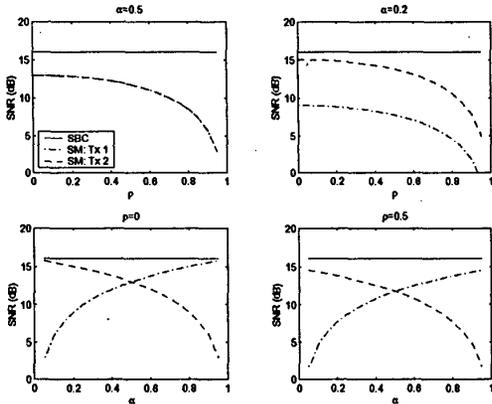
Figure 3. The post processing SNR of the SBC and SM modulators when  $N_r = 2$ ,  $\|\mathbf{H}\|^2 = 4$ , and  $E_s/N_0 = 13\text{dB}$ .
