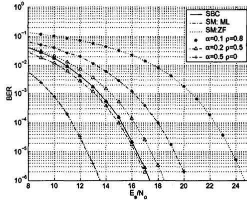
Figure 5. The BERs of the SBC modulator with 16-QAM and the SM modulator with QPSK in fixed channels with different  $\alpha$  and  $\rho$ .
