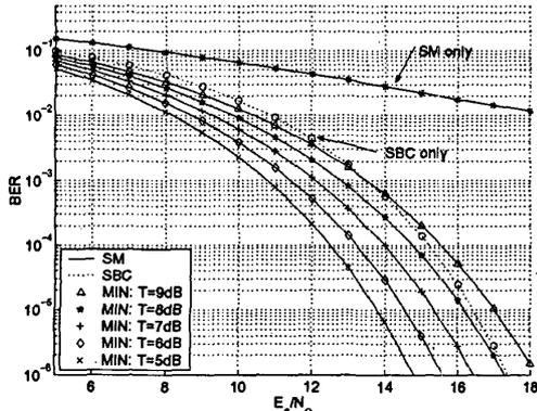
Figure 6. The BERs of the proposed system when the ZF receiver is employed for the SM.
