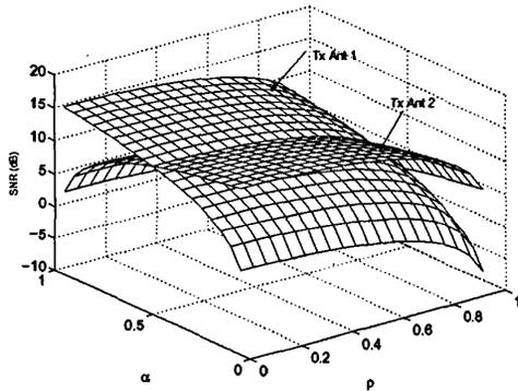
Figure 4. The post processing SNR per transmit antenna of the SM for various  $\alpha$  and  $\rho$  when  $N_r = 2$ ,  $\|\mathbf{H}\|^2 = 4$ , and  $E_s/N_0 = 13\text{dB}$ .
