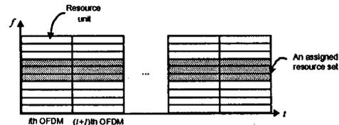
Figure 1. An example of resource allocation in an OFDMA system.
