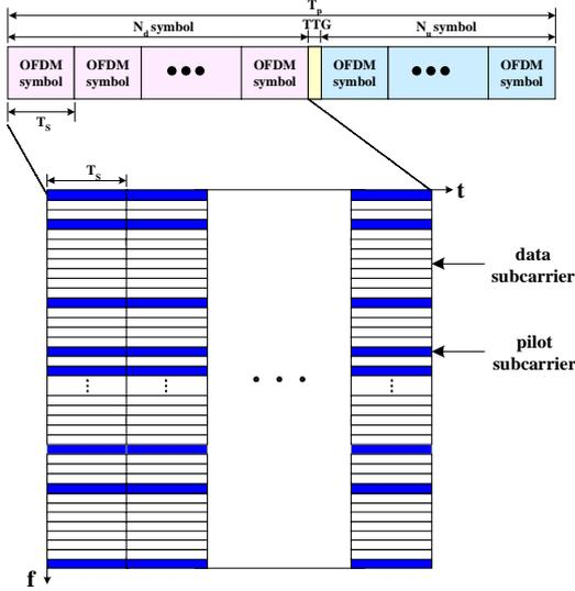
Fig. 1. Frame structure and pilot structure for OFDM(A)/TDD-based cellular systems
