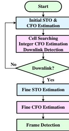
Fig. 3. Flowchart of synchronization and cell searching for OFDM(A)/TDD-based cellular systems
