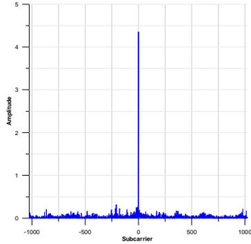
Fig. 4. Autocorrelation characteristic of random pilots (vehicular channel A with 100km/h, SNR: 5dB, normalized CFO: 1.1, STO: -10)
